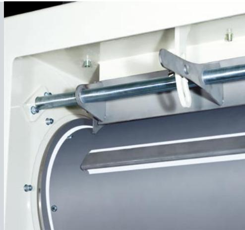
Opened access door showing the drum jacket and the segment-type gate.
