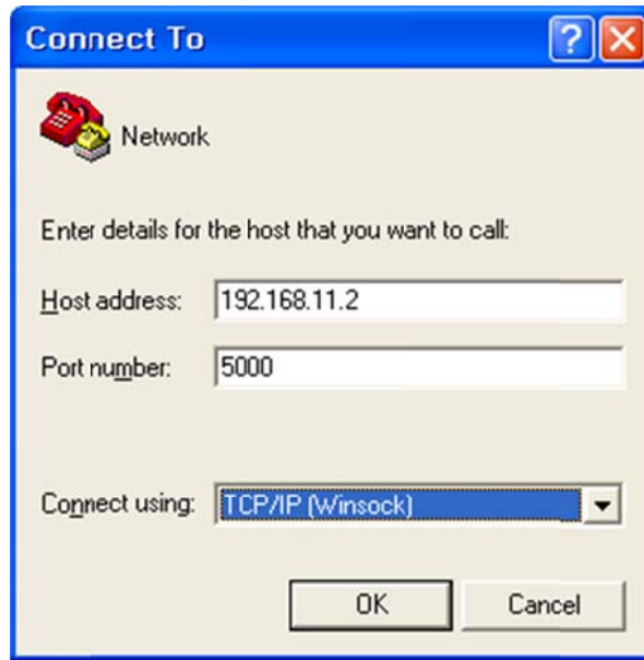
Figure 24. Network Terminal Program configuration
