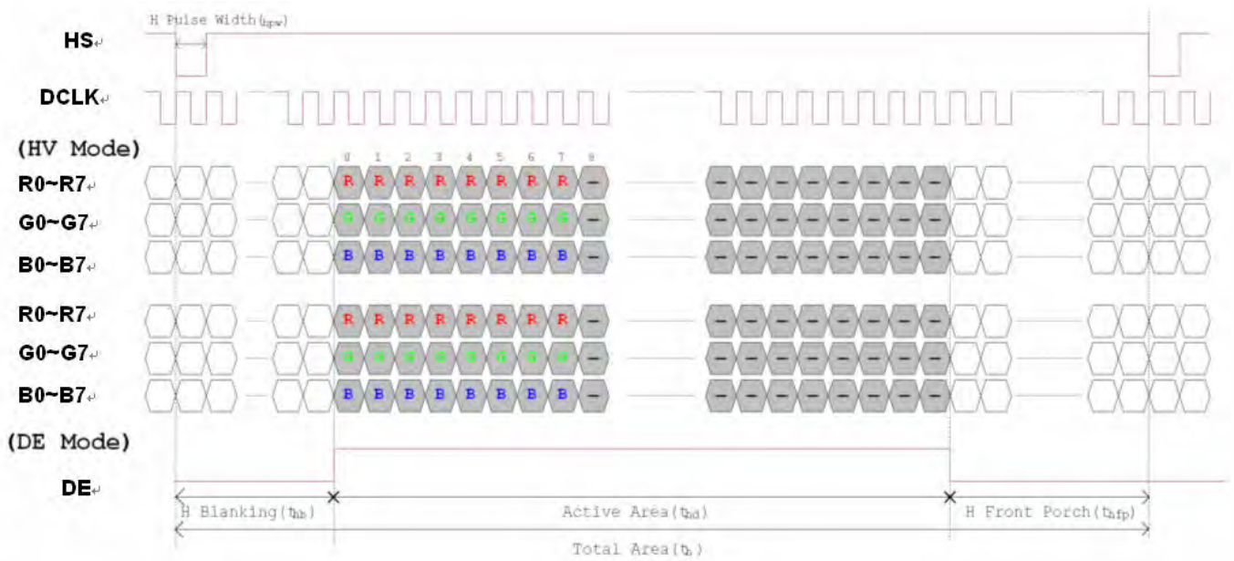
Figure 3. 1 Horizontal input timing diagram.
