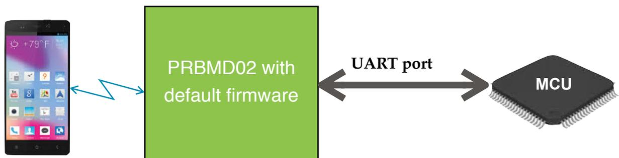
data from BLE appears on UART\_TX pin automatically
