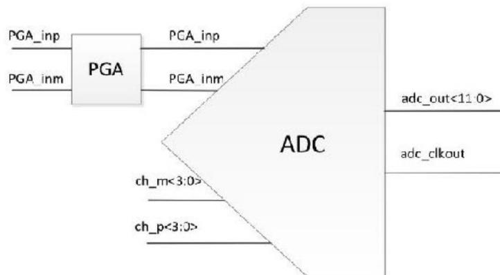
8. PGA provides 42dB gain range from 0dB to 42dB in 3dB steps.
